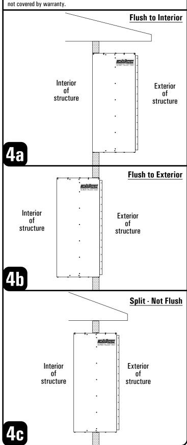
Using a minimum of 12 fasteners suitable to your structure secure the unit in the opening as shown below, 3 fasteners per side.
