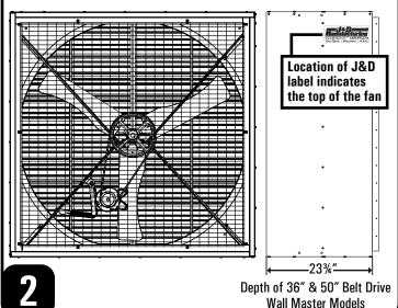
Using a #2 square drive bit remove and set aside rear guard and clips. If installing optional weather hood (not included), wall master must be mounted flush to the exterior as shown in Step 4b.
