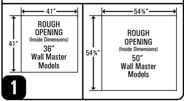
The top of each wall master is indicated by the location of the J&D label on the sides of the fan. Do not mount unit in any position but upright as shown below.
